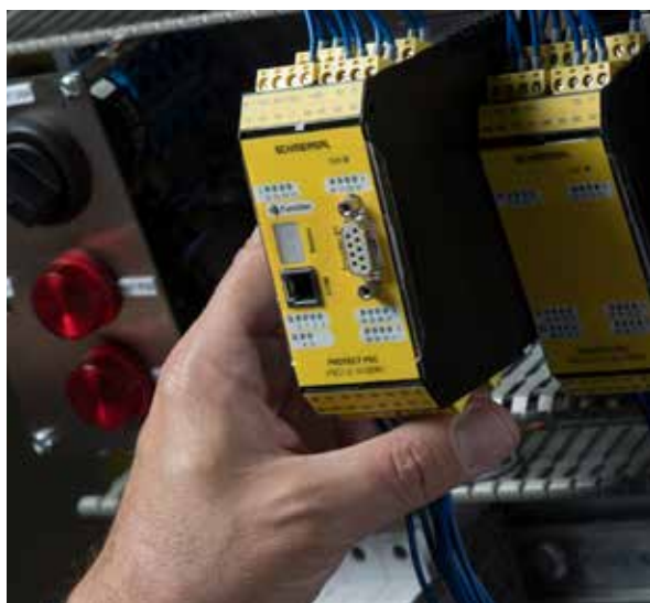
An efficient solution for complex systems: the PROTECT PSC1 safety controller
